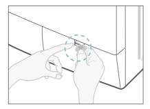
**3.** Unscrew the emergency drain cap by turning left. Grip the cap on the end of the emergency drain tube and slowly pull it out about 15 cm.
